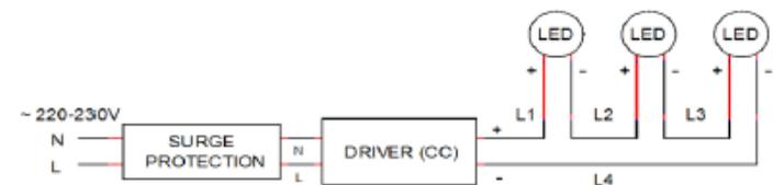
The voltage consumed by a lighting is equal to its power divided by its intensity (ex. : 1,5W / 0,35A = 4,3V).
