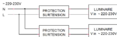
Directly on the single-phase stabilized network (the driver is integrated into the lighting)
