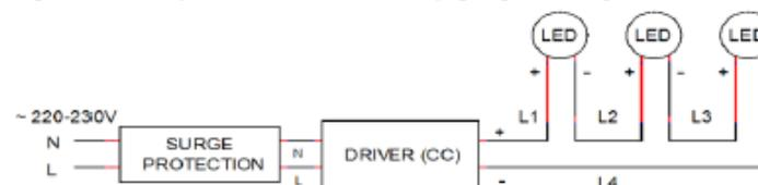
The voltage consumed by a lighting is equal to its power divided by its intensity (ex. : 1.5W / 0.35A = 4.3V).
